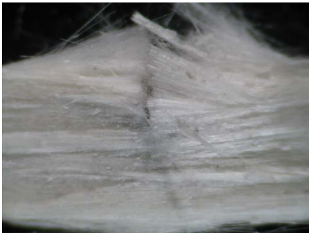
Fig. 6 Typical damage observed during the flexural tests
